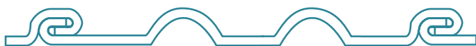
Spiral pipe lock seam (RL-1) (Corrugated 14" and larger for extra strength below grade)
